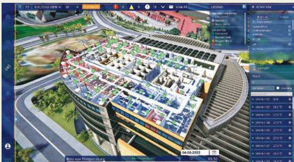
Cross-section of JTC Summit's Digital Twin, showing almost real time data of the cooling system in the building
